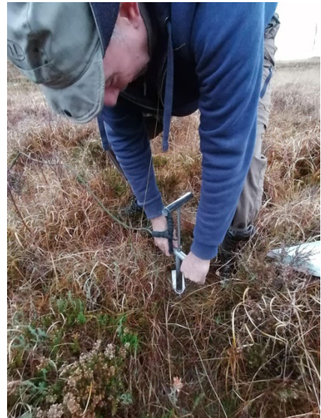
2. T1 location. Peat auger 1m deep. 24-12-2024.
